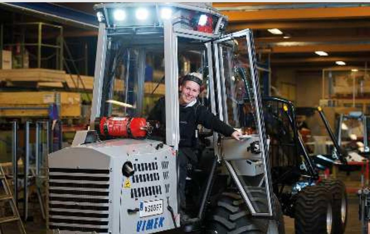
**6** The mechanics test run all forest machines and prepare test protocols. Final adjustments and inspection of the technical functions then take place so as to guarantee that all machines leaving Vimek are quality-tested. All forwarders for the Swedish market are inspected by Svensk Maskinprovning prior to registration and before delivery to the customer. This means that Vimek's forwarders meet all requirements for use on public roads.
