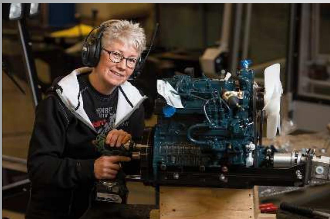
5 The machine frame, motors, tanks, valves and machine cabins are installed during pre-assembly. Then comes the final assembly of all other equipment and technology. The mechanics work in teams of two and build all machines from start to finish. Each machine consists of about 800 different items and it takes about nine working days for an assembly team to build a complete machine.
