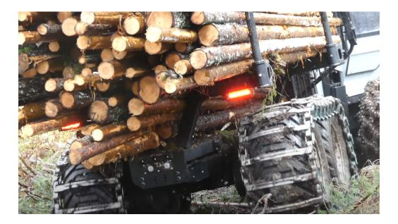
Vimek 870.1 NG has DSS (Dual Steering System), this means steering in both middle joint and rear boggie. This reduce the space required to operate Vimek 870.1 NG in stands.
